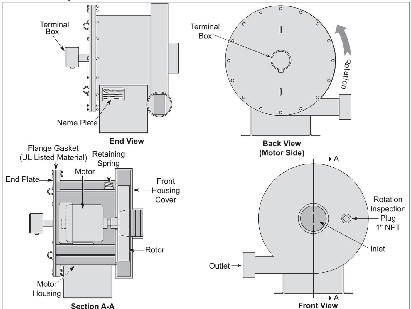
Figure 2. Parts Identification & Location - HB Series
