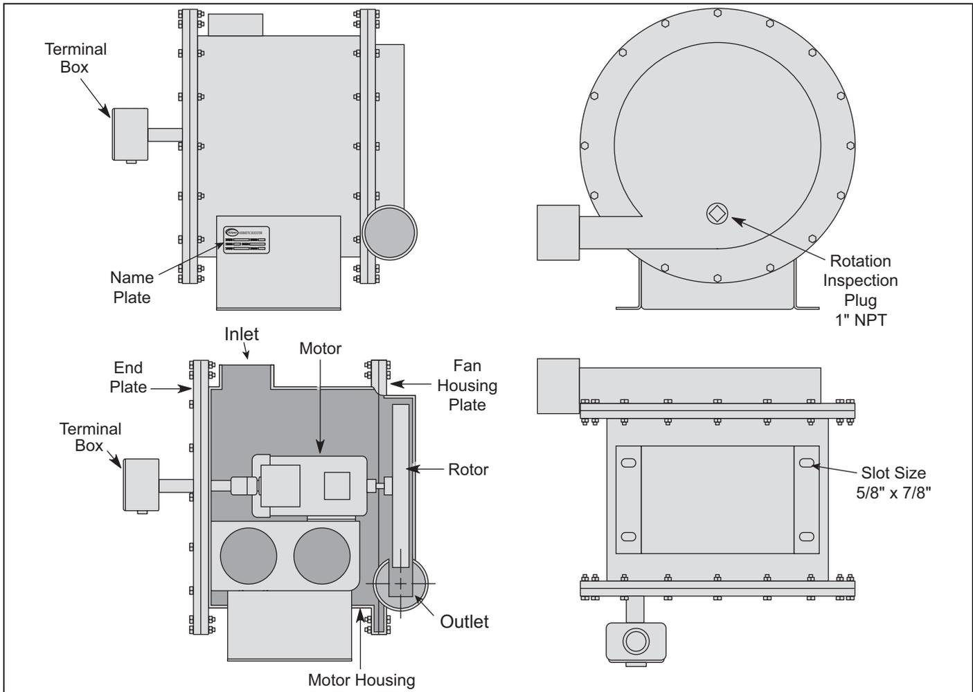
Figure 3. Parts Identification and Location - **HBLC Series**
